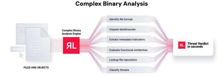
The complex binary analysis process begins by identifying the format of the file or object. Advanced file deconstruction means that once the object is identified, automated unpacking and de-obfuscation takes place with support for more than 400 packer formats (e.g., archives, installers, and compressors) along with the ability to identify over 4800 different types of files (e.g. PE/Windows, ELF/ Linux, Mac OS, iOS, Android, FLASH, media, documents, and more).
